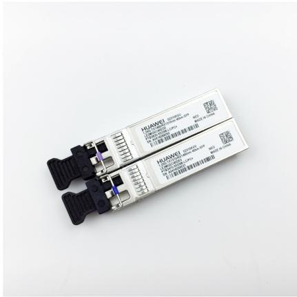
Huawei LE2MGSC40DE0 Optical Transceiver, eSFP, GE, BIDI Single-mode Module (TX1310/RX1490, 40km, LC)
