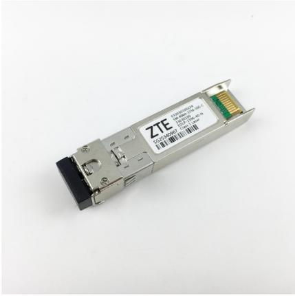
Módulo Transceptor ZTE 10G 1550nm SM 40km C-temp SFP+ EOLP-1596-40-N SPP-10E-ER-CDFA
