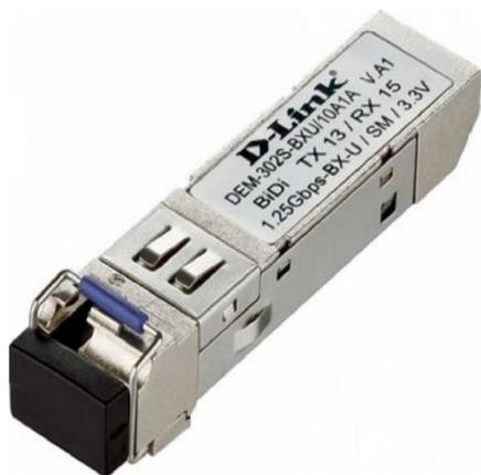
Transceptor D-Link DEM-302S-BXU SFP 1 porta 1000Base-BX para SMF, fonte de alimenta 3,3V (até 2km), WDM (TX: 1310nm, RX: 1550nm)
