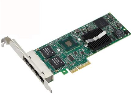
Adaptador de servidor Intel Gigabit ET2 Quad Port, 82576, Gigabit Ethernet, Quad Port, cobre RJ45
