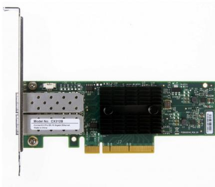
Mellanox MCX312B-XCCT ConnectX-3 Pro EN placa de interface de rede, 10 GbE, porta dupla SFP+, PCIe3.0 x8 8GT/s, suporte alto, RoHS R6
